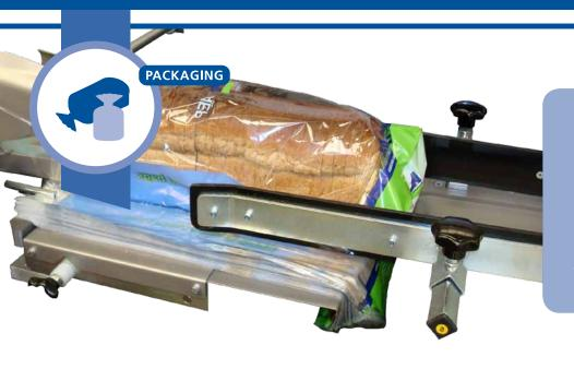
Semi automatic machine for easy bag opening and loading of bread and buns into pre made wicket bags. Possible to combine this machine with a closing conveyor, or to integrate it into the outfeed table of a bread slicer.
