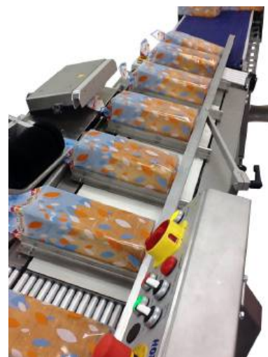
Optional ▶ roller infeed after flowpacker
