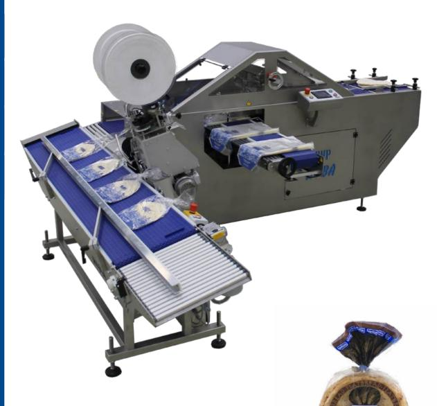
Fully-automatic packing machine HWP for loading flatbread, pita, tortilla or naan bread automatically into pre made wicket bags. The machine has been developed to high quality engineering standards using our knowledge of the national and international bakery markets.
