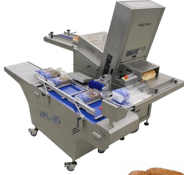
The bread slicer HSA-55 with continuously rotating band blades, angled to pull the loaves smoothly through the blades, with the advantage that they are not pressed together, resulting in optimal slicing results.
